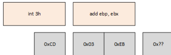
Figure 3.5: Illustration of the incorrect disassembling of "int 3h" by Windbg.
