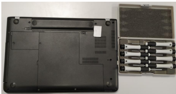
Figure 7.24: Access to the mother board on a laptop.
