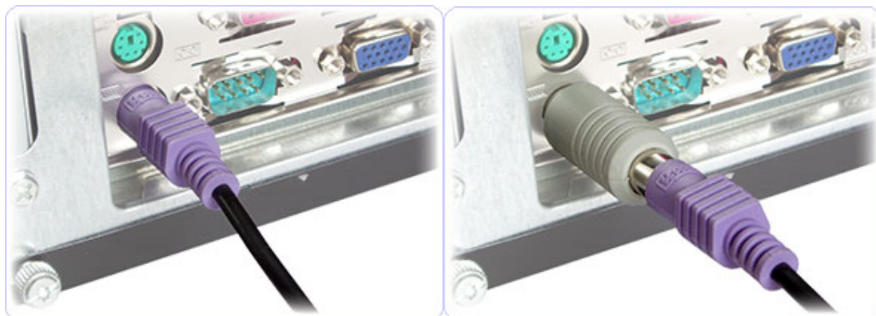
Figure 5.2: Usual connection between PS/2 keyboard and computer. Figure 5.3: Keylogger lies between PS/2 keyboard and computer.
