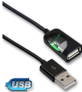
Figure 5.10: Illustration of KeyGrabber Forensic Keylogger Cable from Keelog.
