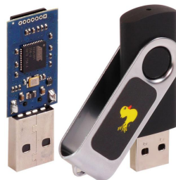
Figure 4.16: Rubber ducky dongle used to emulate a keyboard with pre-recorded sequences of keystrokes. The technologies behind this type of device are direct applications of USB and HID protocols.
