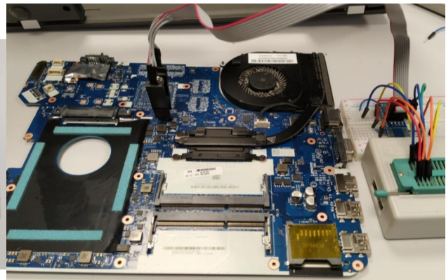
Figure 7.25: Electronic setup for flashing the contents of the machine's BIOS/UEFI.
