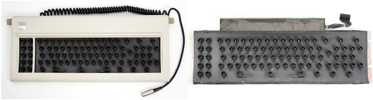
Figure 4.4: Keyboard IBM-PC model F type 1 mechanism from top without key.
