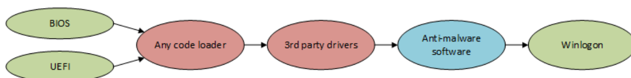
Figure 6.23: Booting procedure before Windows 8.
