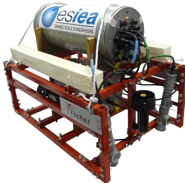
FIGURE 29 – Prototype Aquatis V2.
